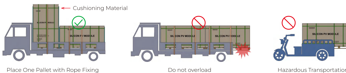
Place One Pallet with Rope Fixing
